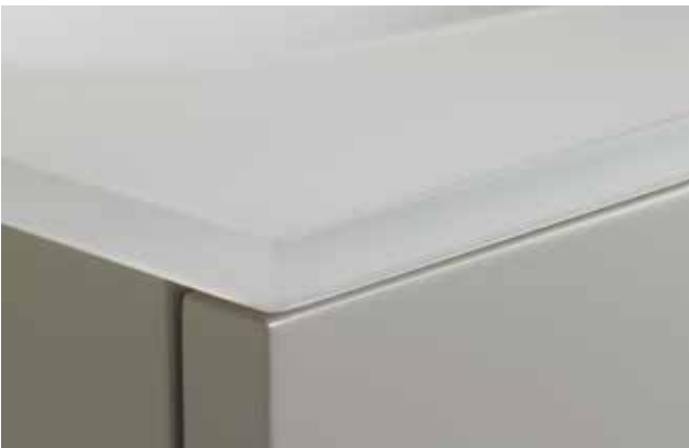
Glide II glass basins are handcast from low iron soda lime silicate glass. Each basin conforms to EN572-9:2005 and EN 14688:2009. Maximum water temperature 70 °C
